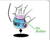
Step 2: Press and hold Evo's Go Button for 2 seconds (or until its top LED flashes white), then release.
