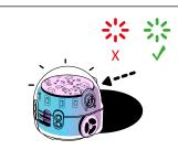
Step 3: Evo will rotate left, right move outside the circle, and blink green when calibrated. If Evo blinks red, start over from Step 2 then release.
