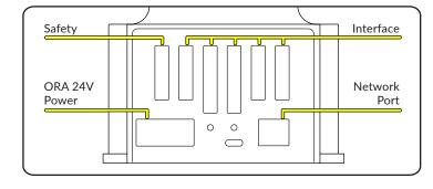
Finally, connect the **Power Supply** and **Ethernet Cable** to their data and power sources. See the figure below for an overview diagram of hardware connection.
