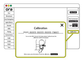
For calibration, you will need the End Tool: Gripper and Calibration tool. See page 24 for connecting an end tool.
