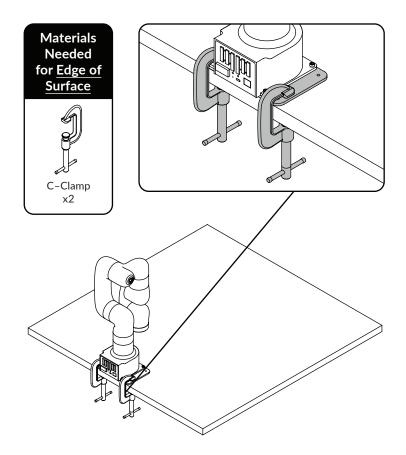
For attaching to an edge of a surface — with half the quadrant mat: connect the top half of the ORA Quadrant Mat together around the base of your ORA, using the two half mat end pieces.
