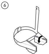
Fold the flaps over the inner portion of the forks.
