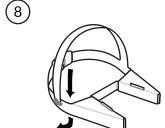
Hook the top strap into the corresponding slot on the other side of the main belt, starting at 90 degrees.
