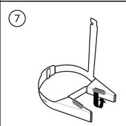
Double the flap over the inner fork and tuck the tab in through the slot to hold it in place.
