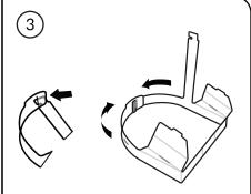
Rotate the hooked side of the belt up. Hook the two ends of the back belt together.
